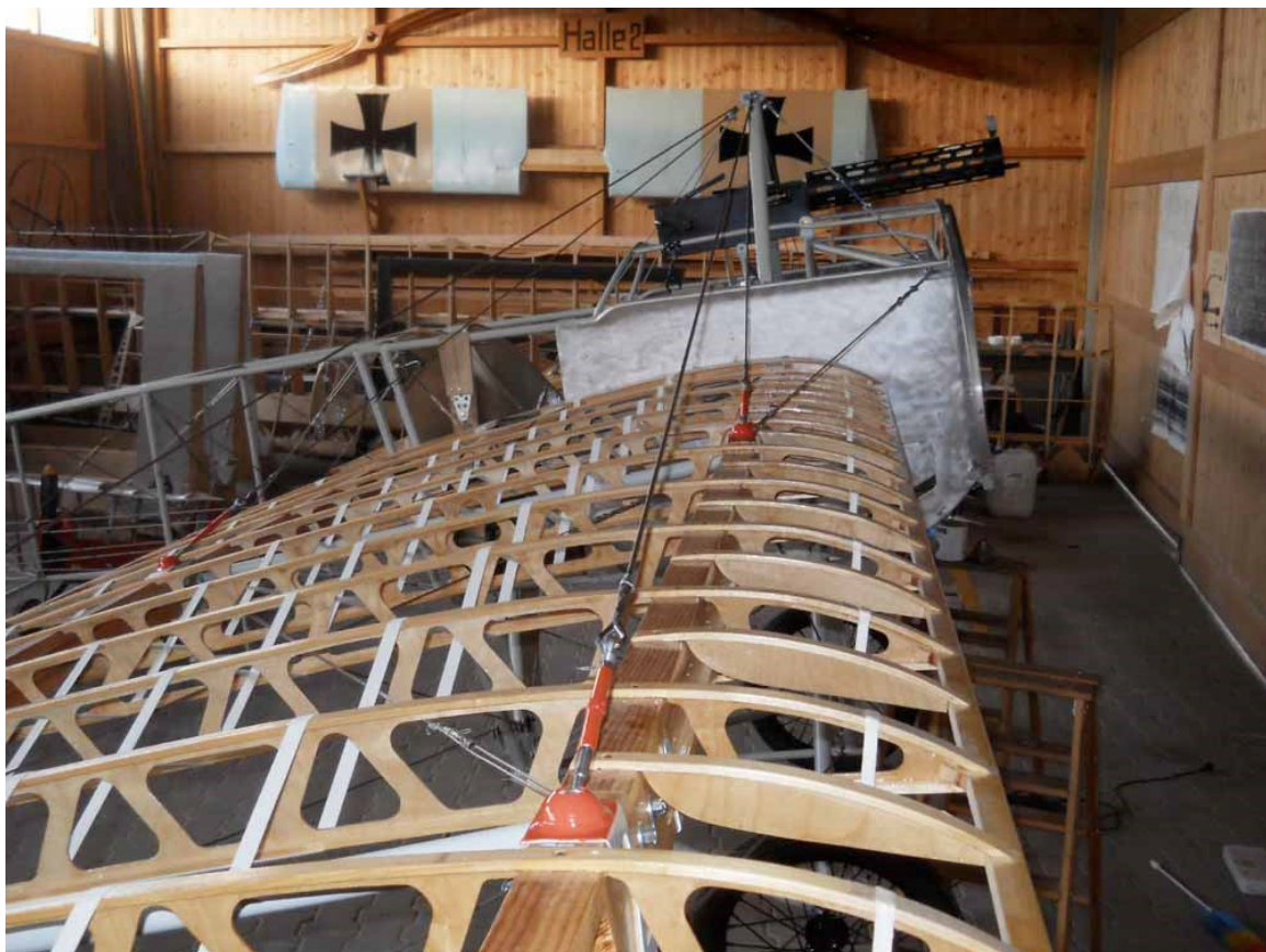
Images of my own E.III showing the differently coloured turnbuckles. Loosening the blue ones allows the red ones to be unhooked.
