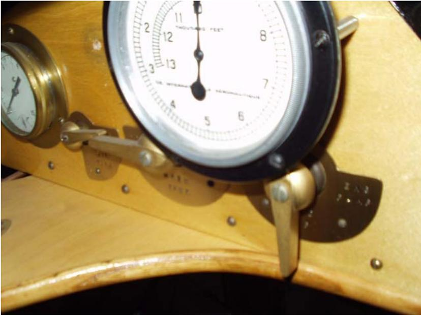
67. Close-up of the altimeter and fuel selector switches.
