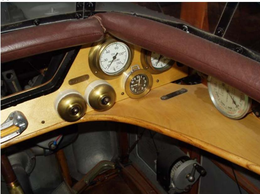
69. Starboard side instrument area, showing the oil pressure gauge, clock, water temperature gauge and tachometer. The two round switches are the mag switches.
