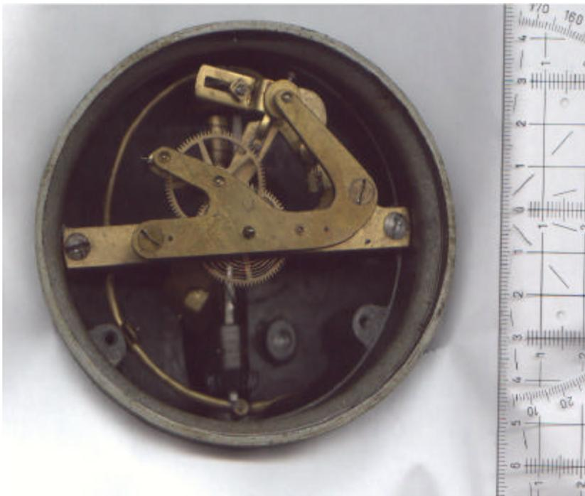
Above, view inside the Phylax after the front face was removed. What is visible at the front is the pointer drive gear. Most pieces of the inner workings are made up from brass.
