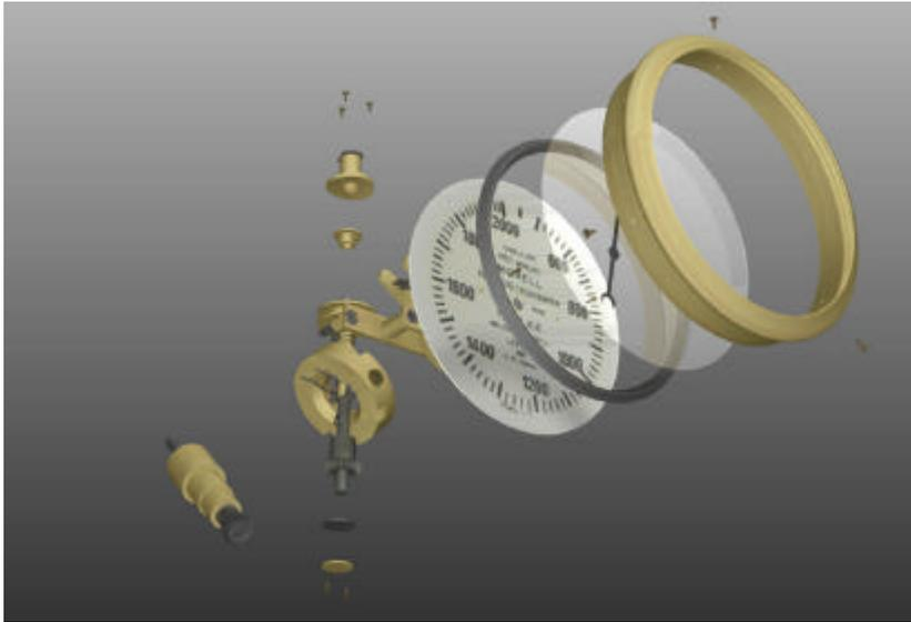
Above and centre, two more exploded views. The one in the centre illustrates how the front portion of the instrument is put together. After the pointer drive is fixed inside the housing by two screws, the face is screwed to its front using two very tiny screws. The pointer now has to be pushed onto the centre axle. The inner front ring is pressed onto the face by the glass which is fixed by the outer front ring.
