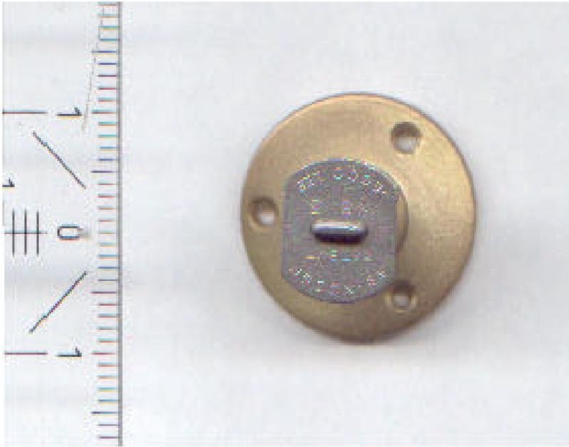
Above, centre and bottom, this illustrates the top oil filler which is made up from brass. The filler cap is made from steel and is fixed to the part by a small chain which is spring loaded so that the cap is always closed. To fill in the oil you have to pull the cap away. The most interesting feature of this the fact that after cleaning it was discovered that this piece was produced by a foreign company and imported to Germany. Closer Details can be found in the text.
