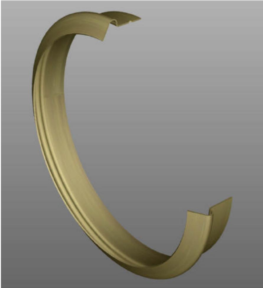
Above, 3D image showing the profile of the pressed brass front ring.
