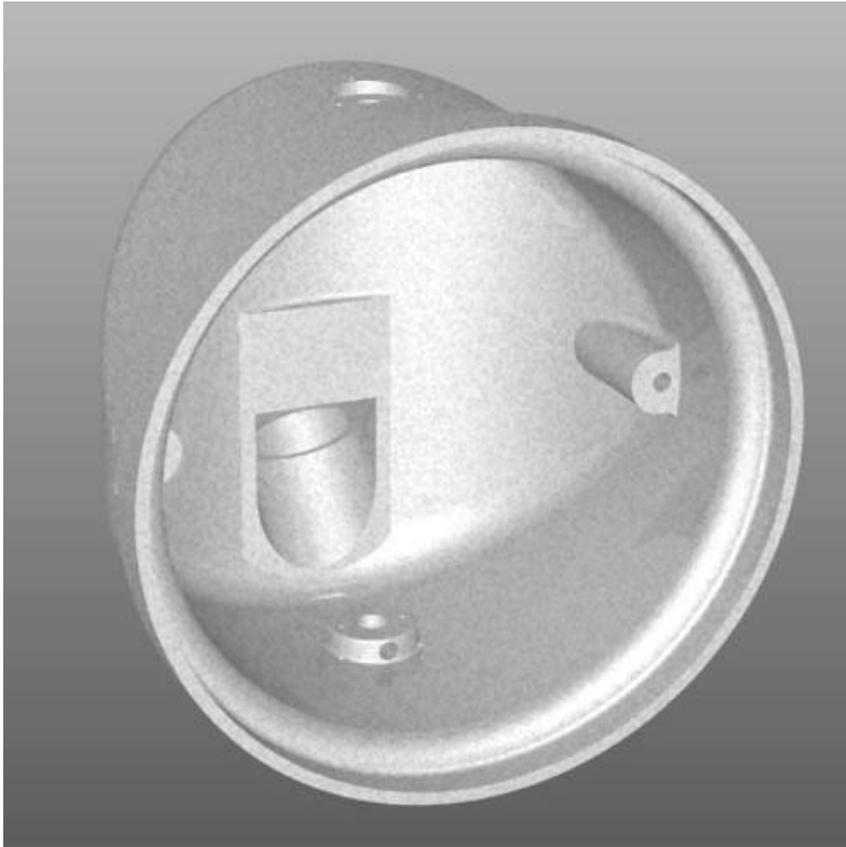
**Above, perspective 3D view inside the housing. As already mentioned this one is made up from rough aluminium casting. In our model we have not incorporated the two bottom fixing pieces that can be seen in the photographs. We do simply not know what they are for. Possibly these are just remains of a earlier design of a gear that was installed in a earlier version of the PHYLAX.**
