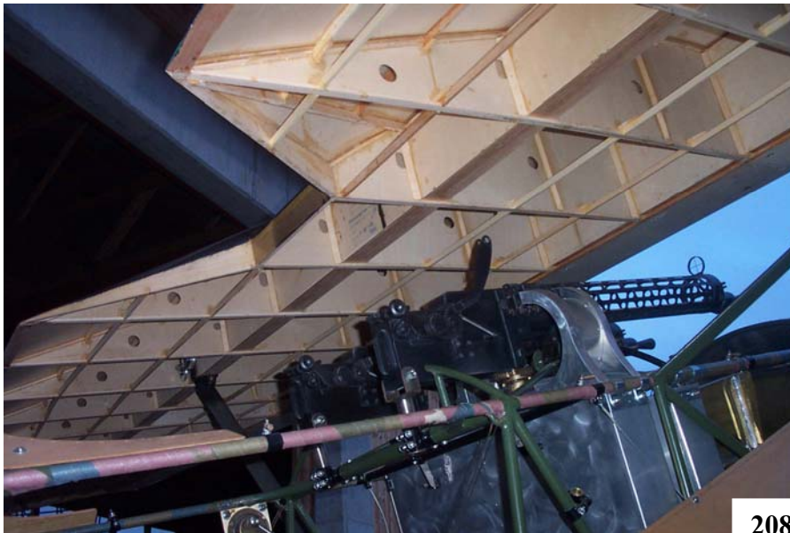
207 and 208. Test assembling of wing and fuselage.
