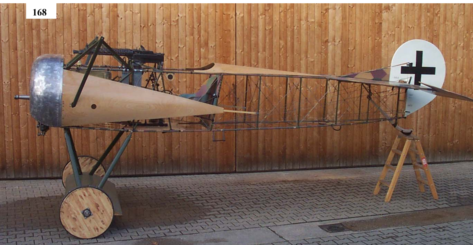
167 – 169. Fuselage with engine cowling and fuel tank in place.
