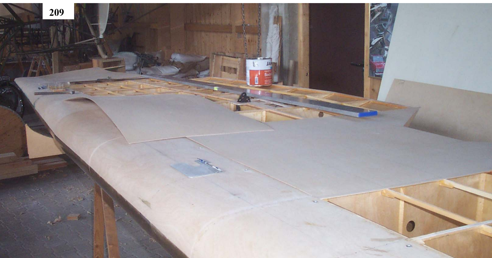
209. The last step is the closing of the bottom side of the wing.
